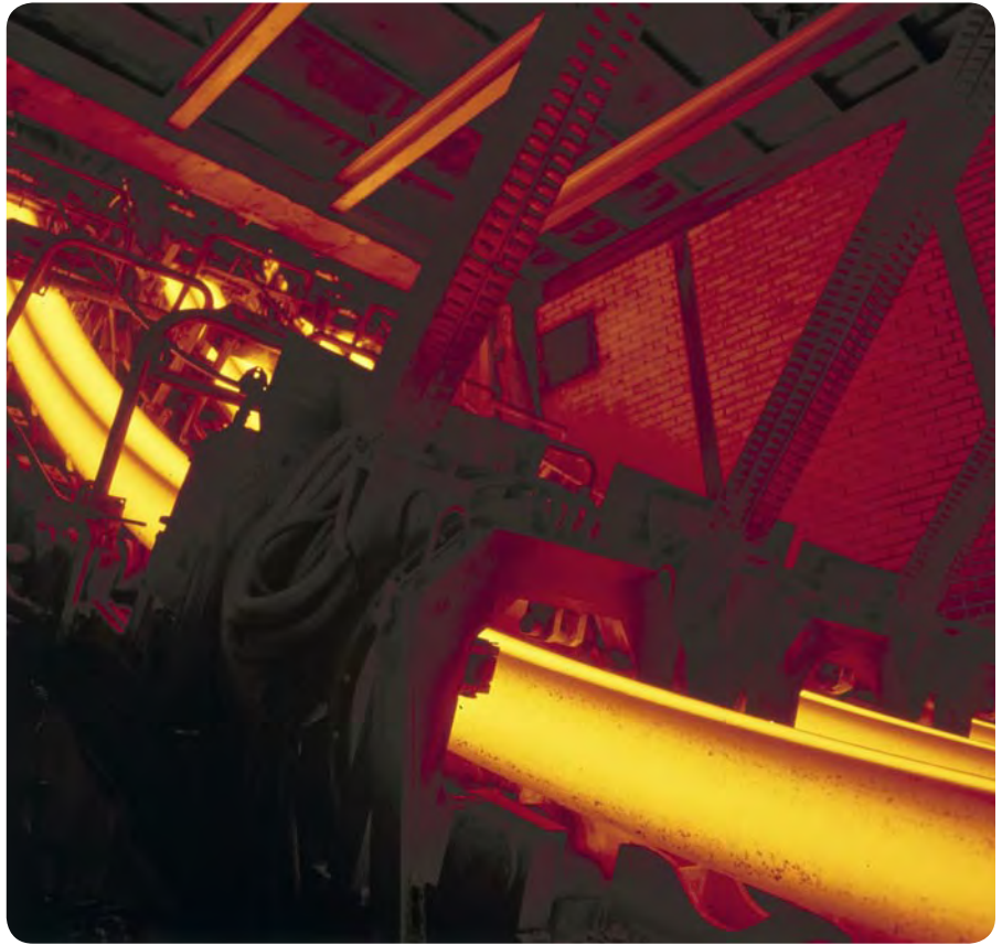
SKF DryLube bearings in the metal industry. Spherical roller bearings or deep groove ball bearings in rolls of continuous casters.
